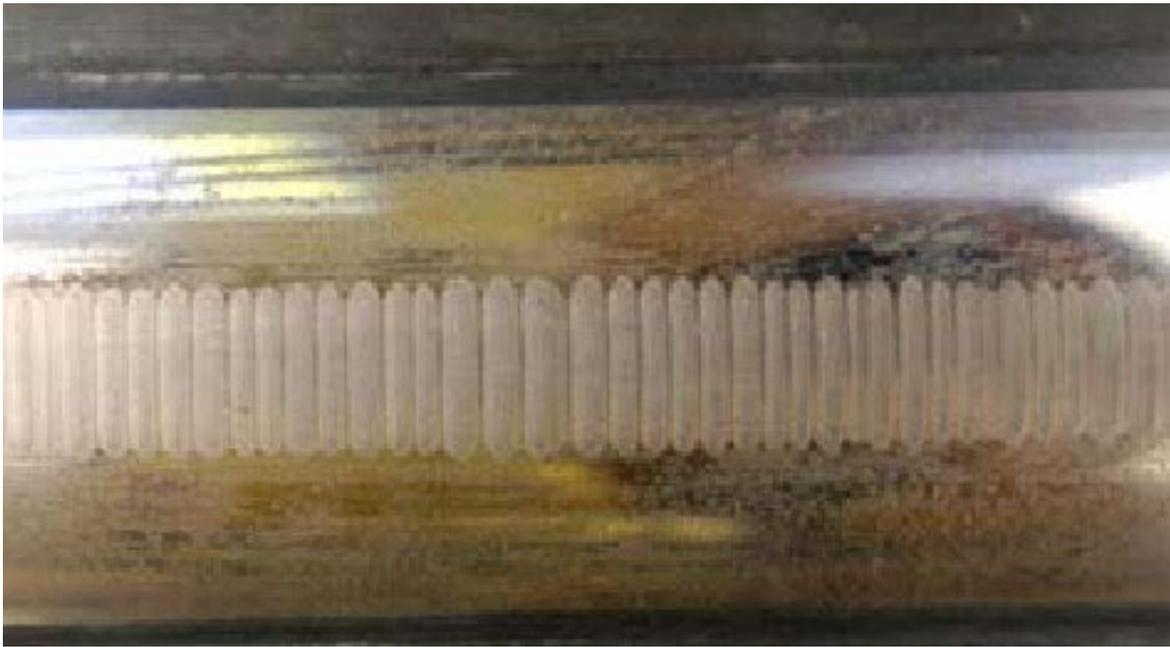
**Figure 27 : Example of “fluting” due PWM VFD common mode current at the switching frequency of the VFD**
