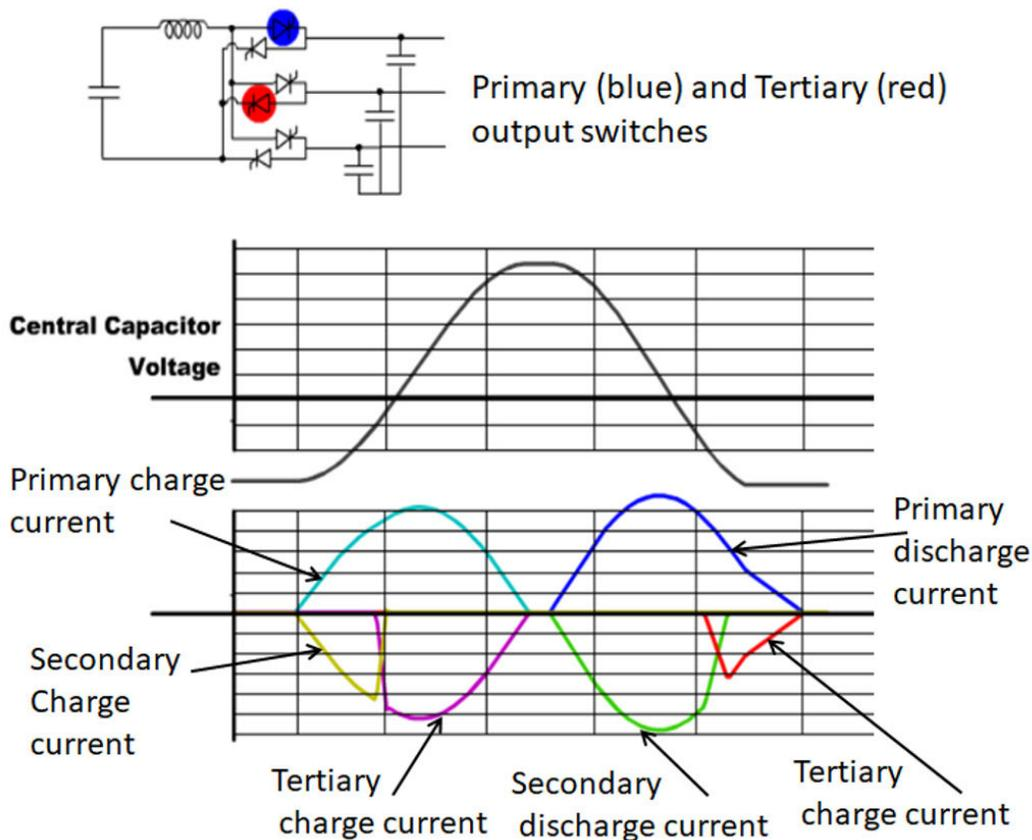
Figure 7 : Resonant Link converter charge and discharge operation
