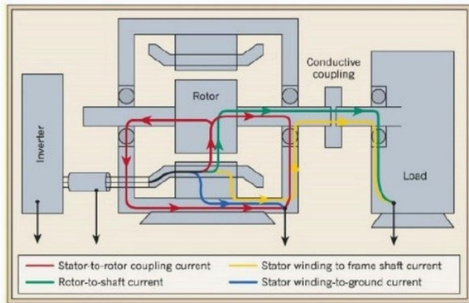
**Figure 25 : Paths of common mode current in PWM VFD fed induction motors**
