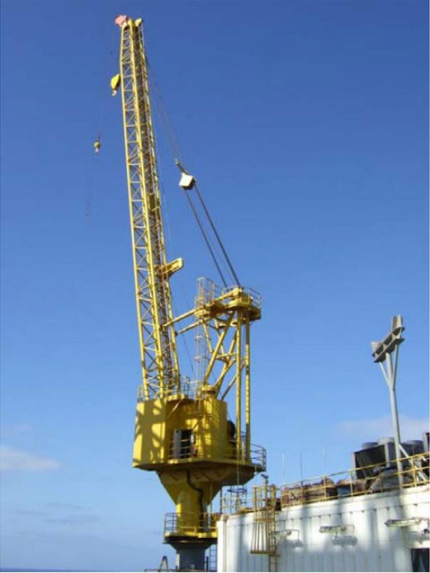
**Figure 23 : Three large cranes on new drilling rig out of action (and off contract) for 5 months due to common mode voltages from draw-works (2 x 1500kW) and top drive (900kW) VFDs**
