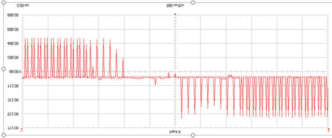
*Figure 19 : Expanded PWM VFD output voltage waveform*
