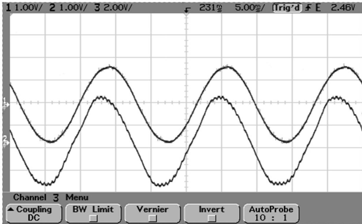
**Figure 8 : Typical input voltage (top) and current (bottom) of 250kW Resonant Link converter.
