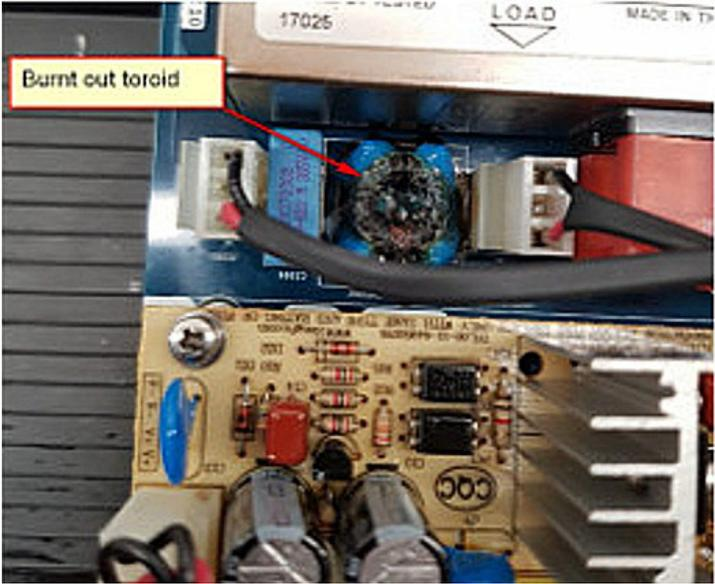
**Figure 24 : Transformer burned out by common mode voltage in US\$ 20,000 MIL spec PQ recorder by the AFE VFDs shown Figure 6. The CMV entered via the single-phase recorder mains supply.**
