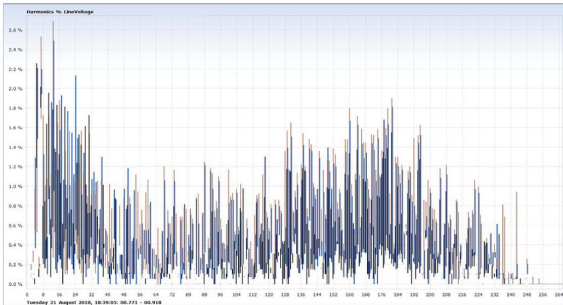
**Fig 16 : Harmonic line voltage spectra of a 500kW AFE VFD (restricted to 256<sup>th</sup> order) at reduced loading (332kW)**
