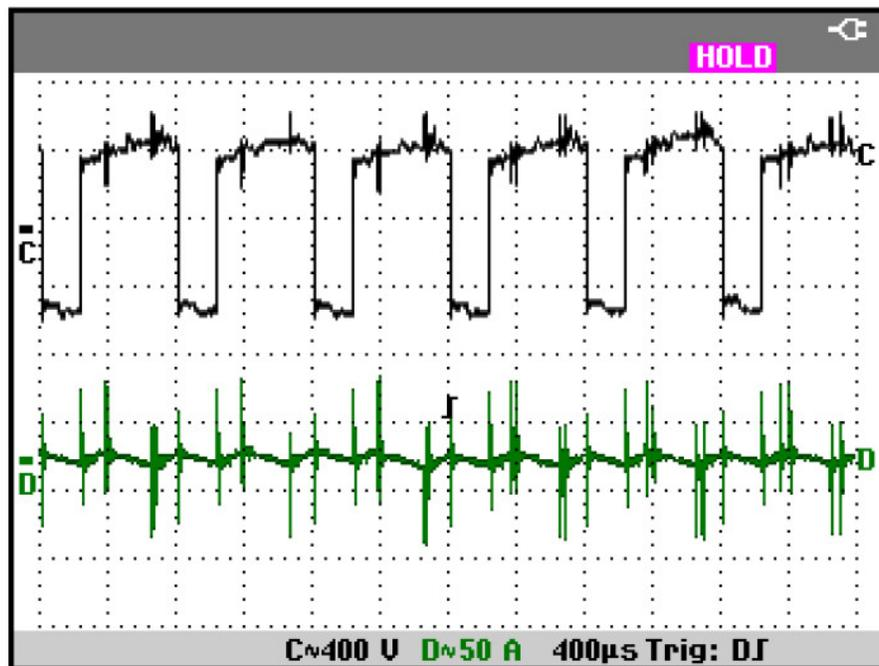
**Figure 26 : Example of common mode current (green trend).
