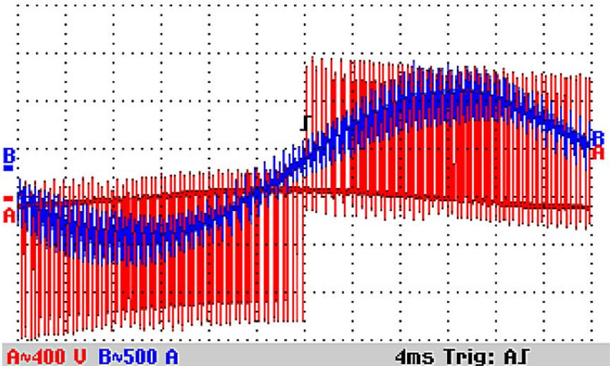
*Figure 18 : Characteristic output voltage and current from PWM VFD*
