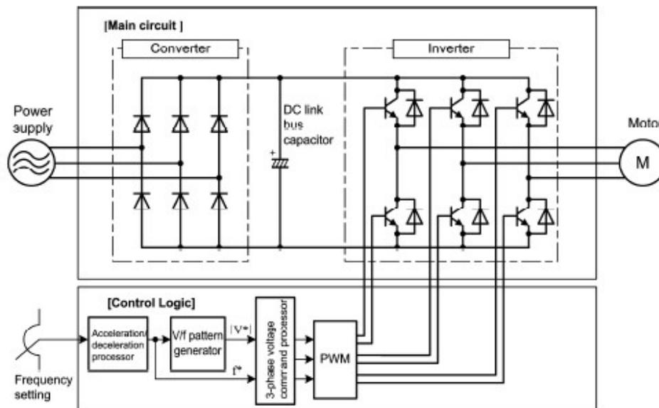
**Figure 1 : Typical 6 pulse PWM VFD**
