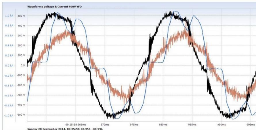
**Figure 12 : Example of a 560kW, 6 pulse PWM VFD input voltage, common mode voltage and phase current using advanced cycle by cycle PQ recorder**
