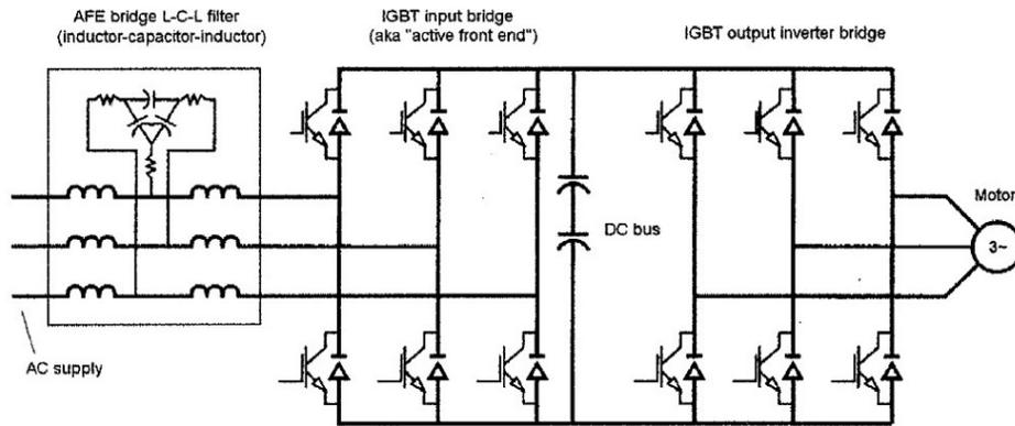
**Figure 2 : Typical simplified schematic of AFE VFD**
