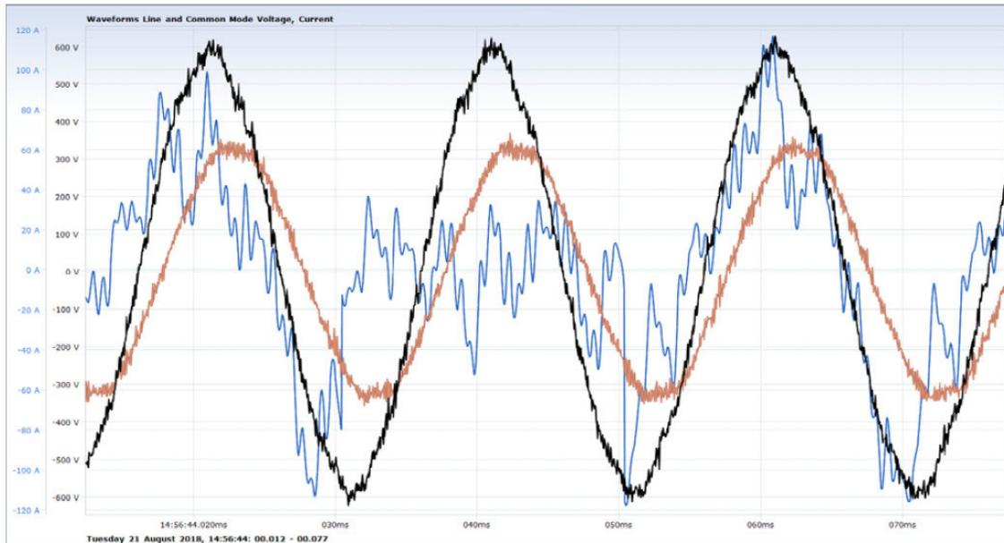
**Figure 15 : Input voltage and current from 500kW AFE VFD at reduced load (332kW). Note the high frequency content of the voltage waveforms and non-sinusoidal and unbalanced nature of the phase currents.**
