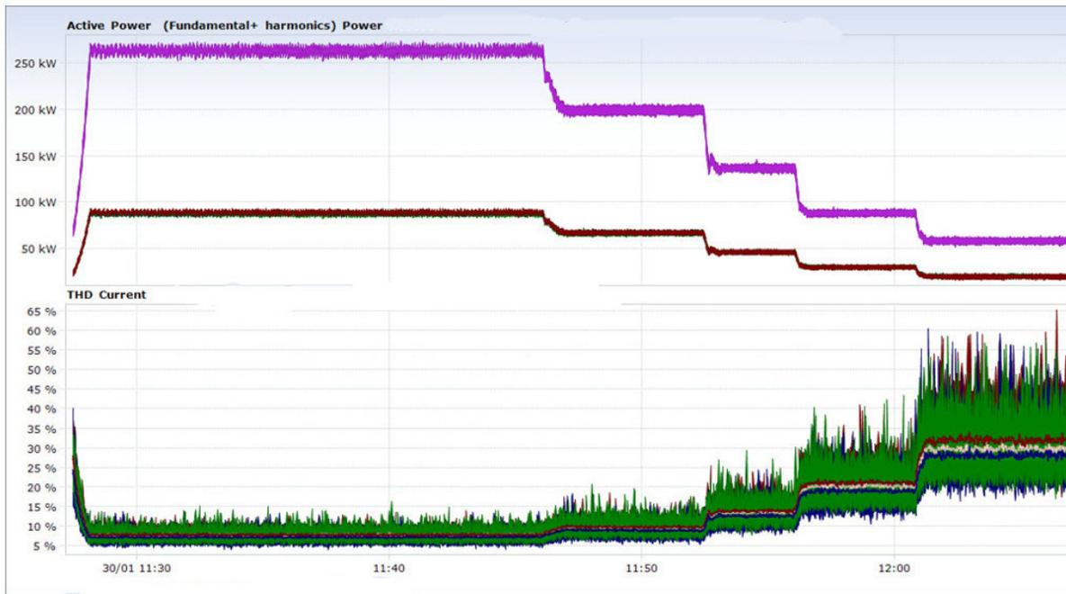
**Fig 17 : Active power (kW) and THDi (average and min/max) of 315kW AFE VFD on centrifugal pump application**
