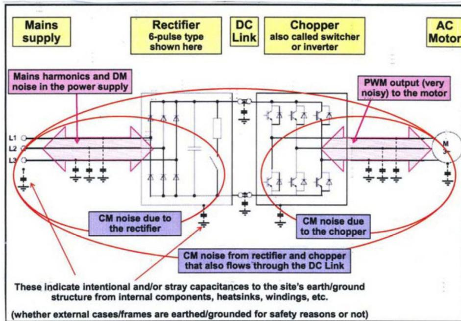
**Figure 20 : Salient paths of EMI in 6 pulse VFD (AFE VFDs have IGBT rectifier)**
