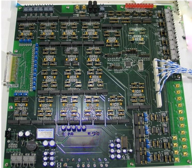
**Figure 11 : Resonant Link converter instrumentation board**
