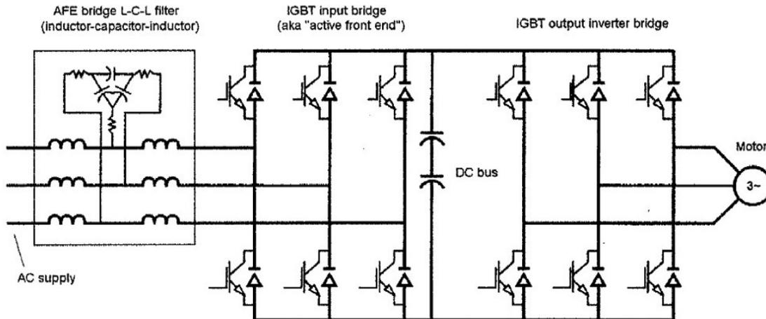
**Figure 14 : Typical simplified schematic of AFE VFD**
