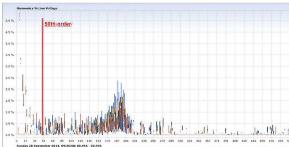
**Figure 13 : The line voltage spectrum of a 560kW PWM VFD during heavy loading (from Figure 12).**
