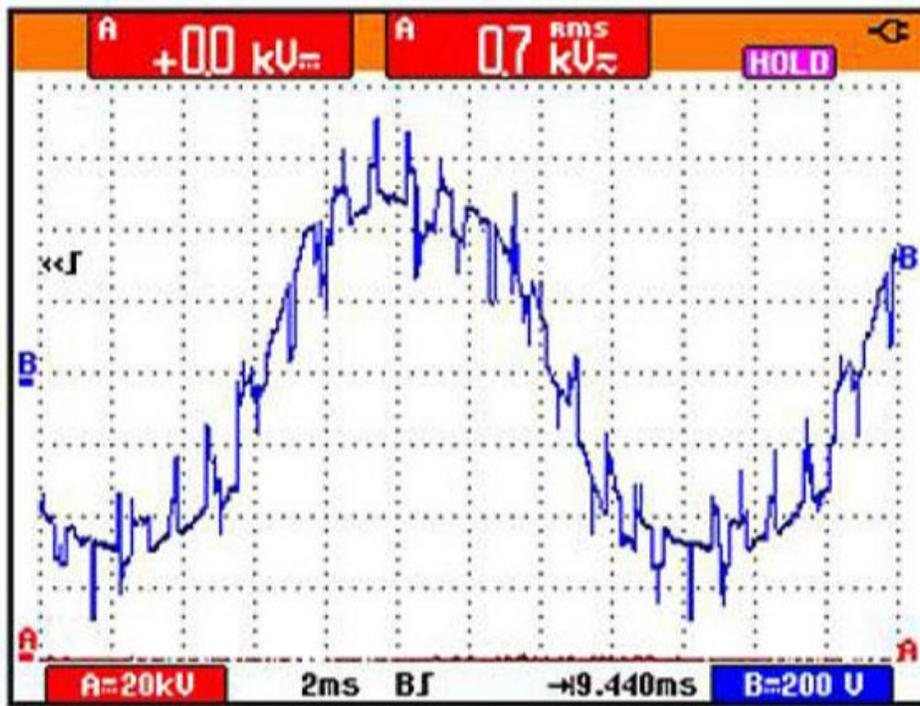
Figure 21 : Example of common mode voltage (1.26kHz switching frequency)
