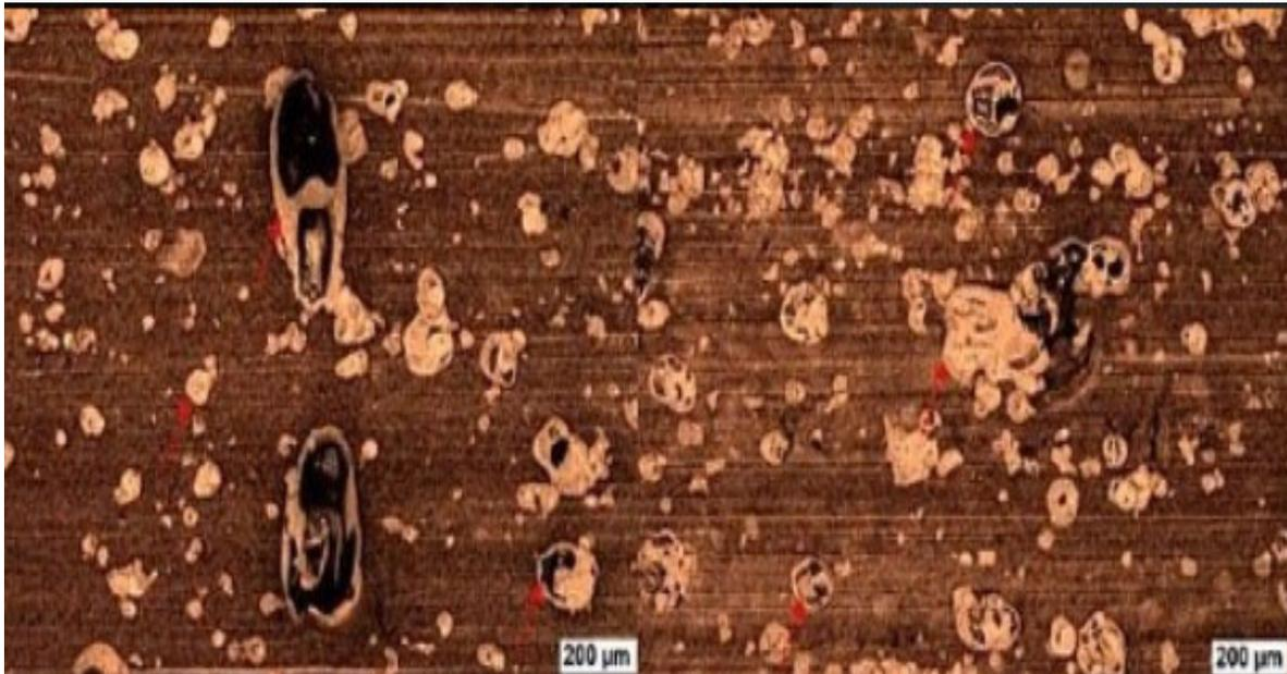
**Figure 28 : Example of “pitting” on 6.6kV EExd fixed speed motors due to common mode voltage emanating from 45MW of PWM VFD main propulsion on an LNG carrier marine vessel. Bearing life was <1400-1600hrs. This problem was common across all 15 vessels in the same class. It also presented a serious safety hazard.**
