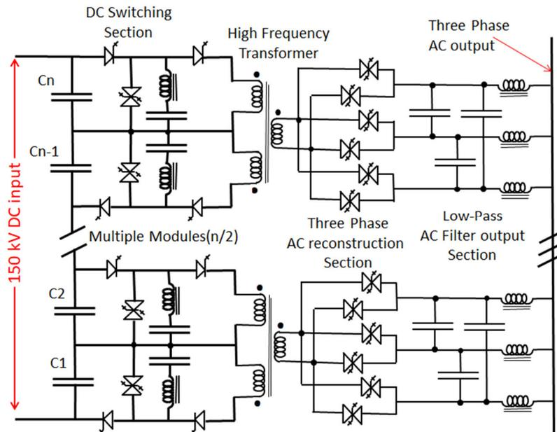
Figure 11 : Resonant Link converter schematics for 150kVDC to three-phase AC reconstruction
