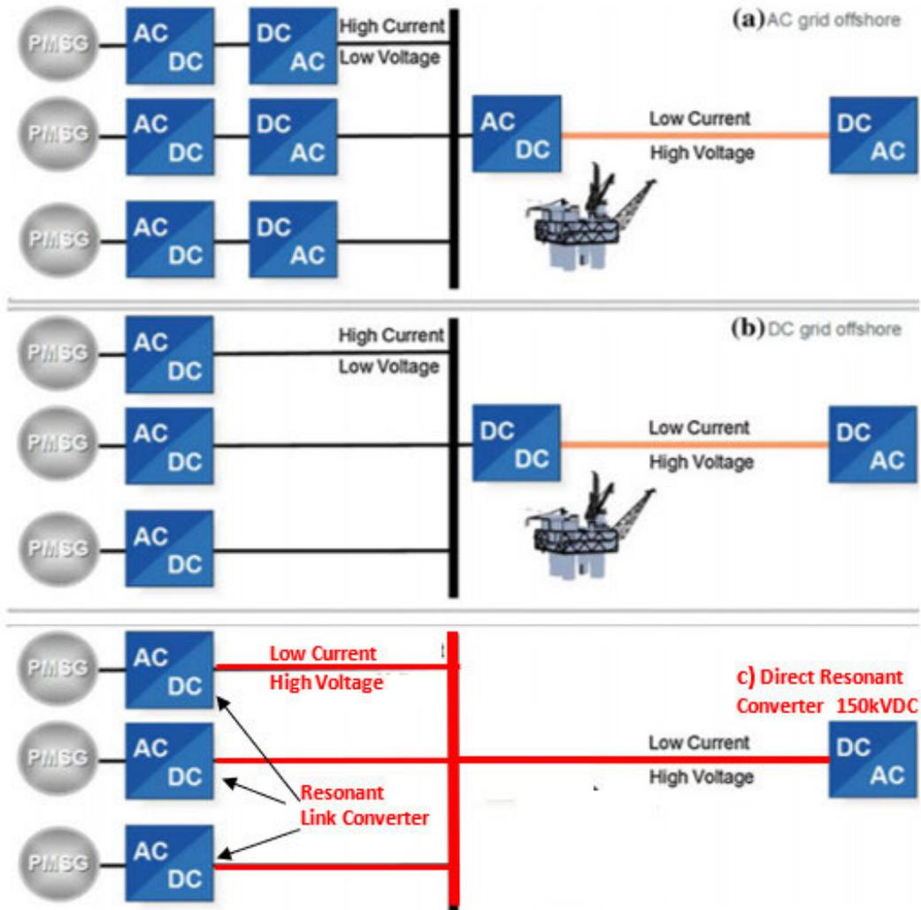
**Figure 2 : Three HVDC alternatives for powering floating wind farms.**
