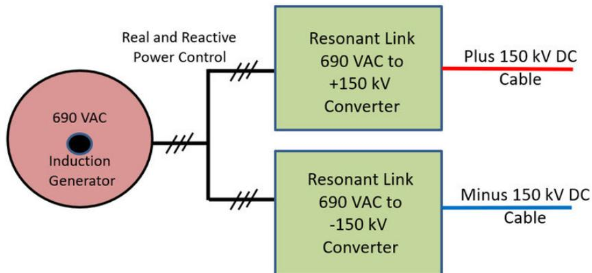
**Figure 5 : Resonant Link topology for 690VAC induction generators**
