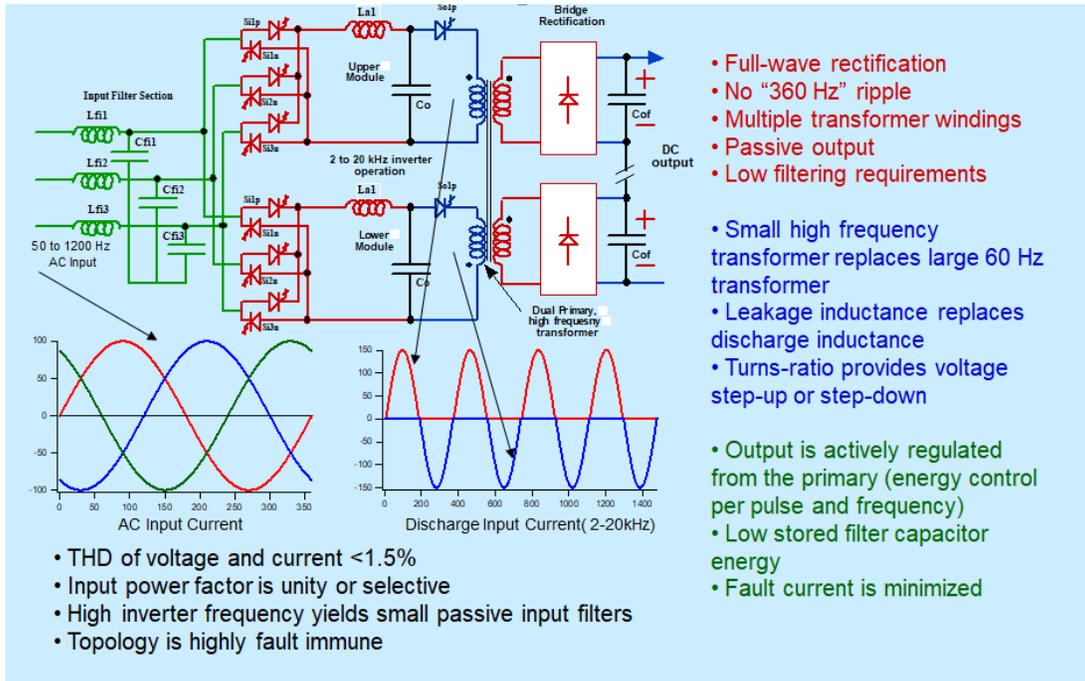
**Figure 3 : Resonant Link AC to HV DC converter
