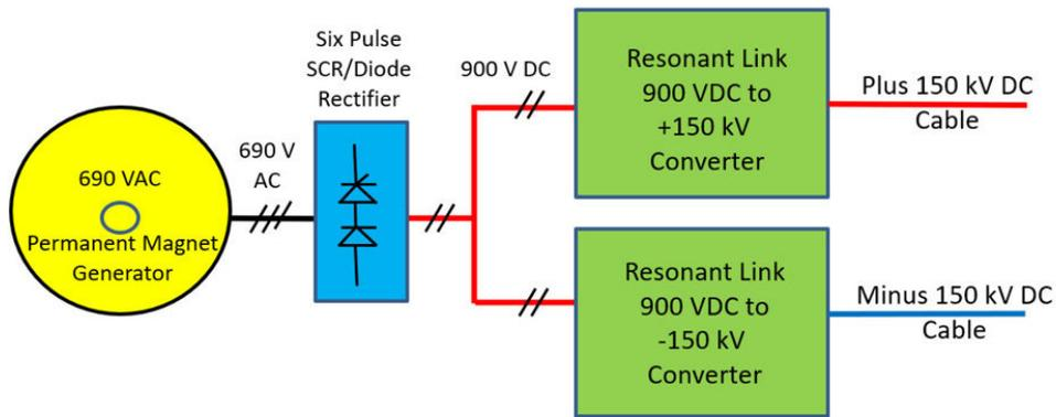
**Figure 4 : Resonant Link topology for 690VAC permanent magnetic generators**
