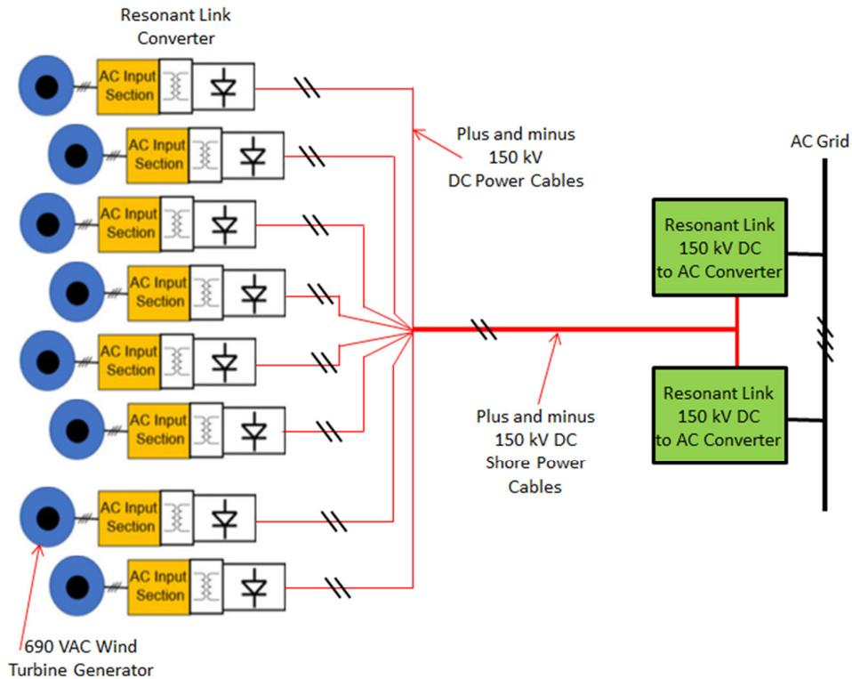
**Figure 9 : Resonant Link Wind Power Generator to 150 kV DC cable transmission to shore DC to three phase AC power conversion**
