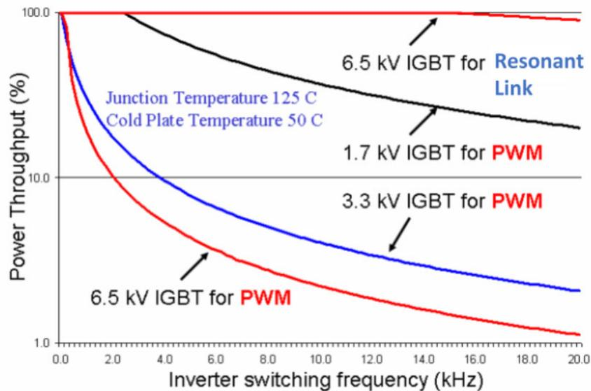
**Figure 10 : Power throughput versus switching frequency of i) IGBT hard-switched PWM converters and ii) soft-switched Resonant Link converters.**
