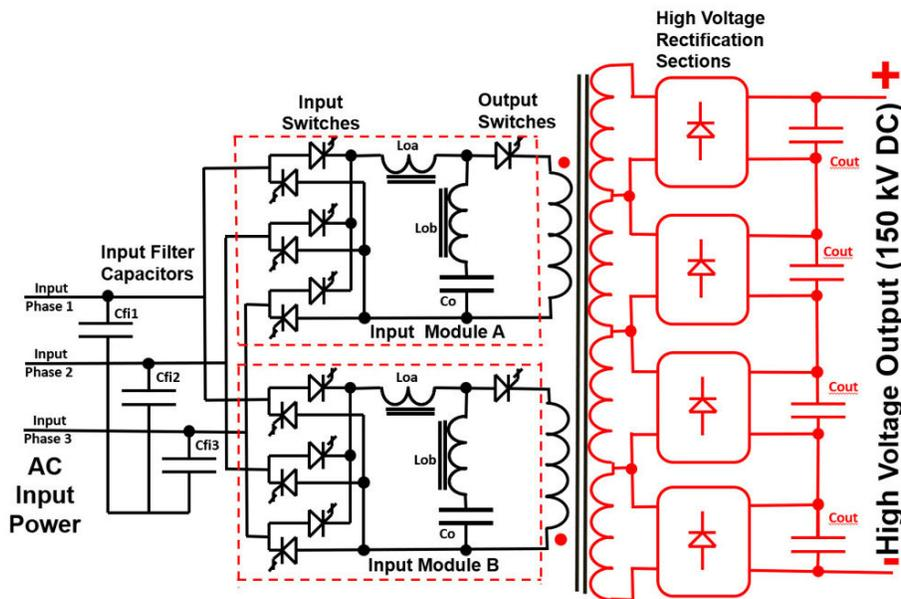
**Figure 6 : Typical 2.5MW, 690VAC to 150kVDC Resonant Link modules (individually plus and minus 150kVDC), are paralleled to match the generator power output**
